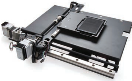
Customised XYZ positioning table
